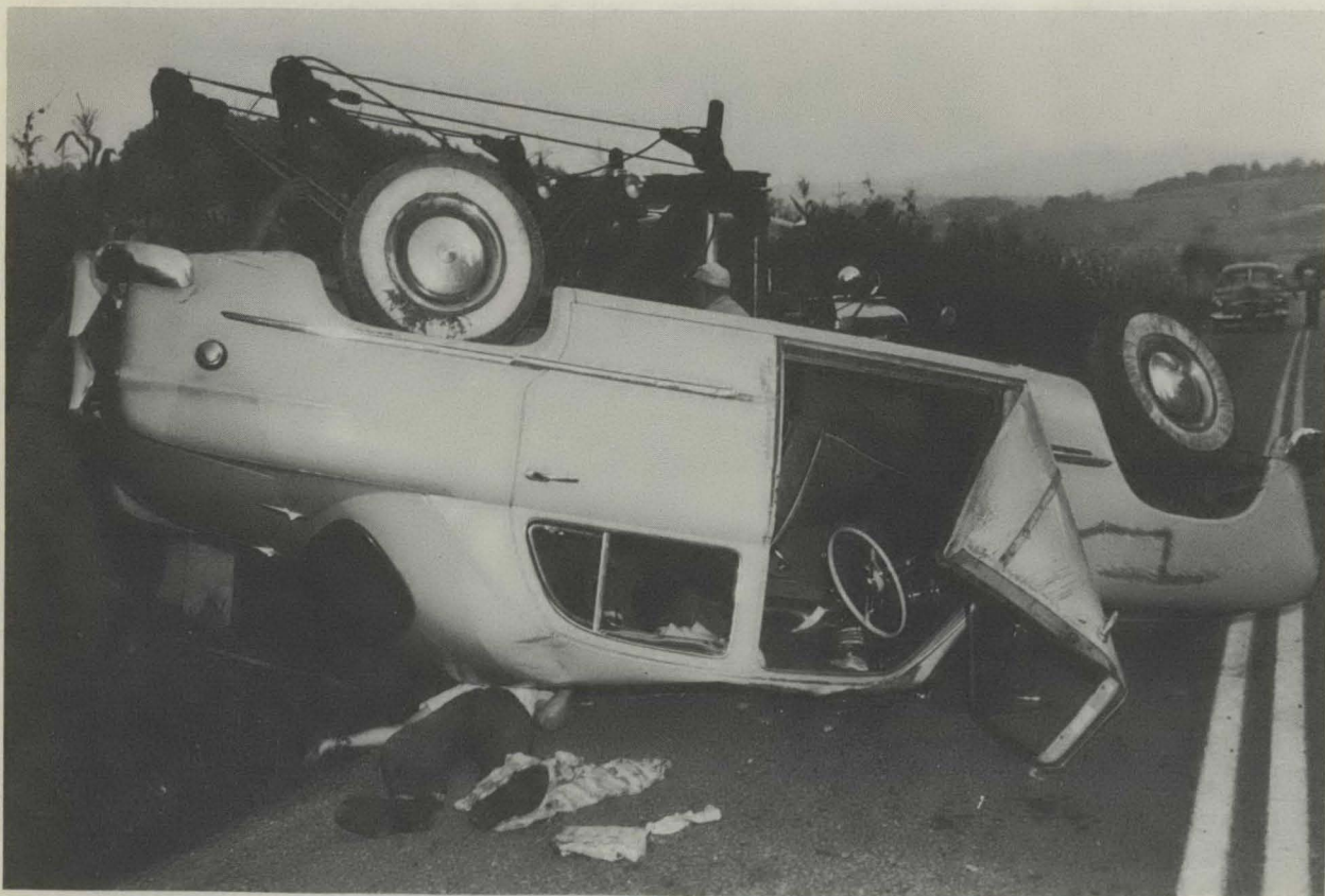
A safety belt would have been advantageous for above driver who was ejected and crushed by vehicle. Note negligible damage in area of driver's seat.
