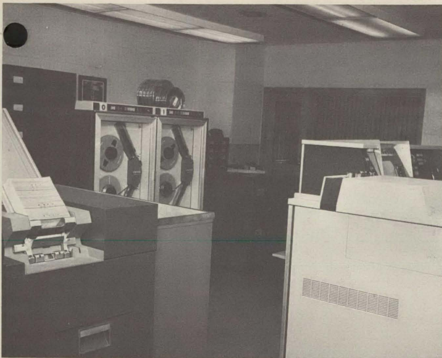
View of computer room showing 088 Collator in left foreground and the UNIVAC 6C Magnetic Tape Transport which is coupled under the floor to the UNIVAC 1004 Processor in the right foreground.
