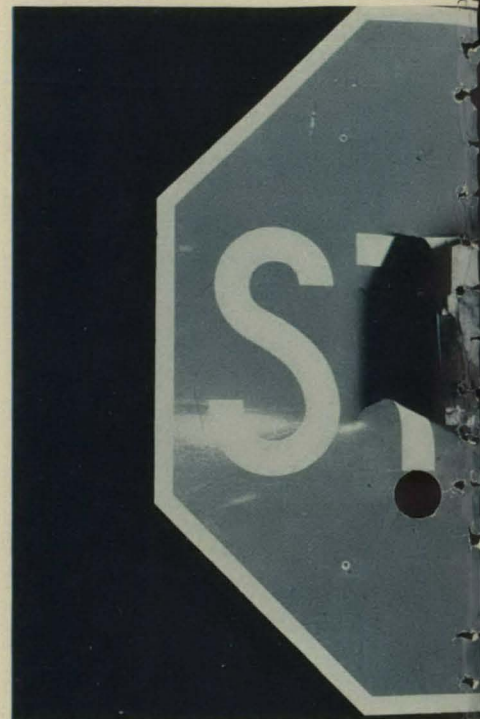
Closeup shows the effects of nitroglycerin on an aluminum stop sign.
