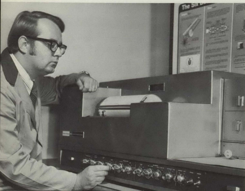
The spectrophotometer, used to identify and compare dyes, measures color and makes a graph.
