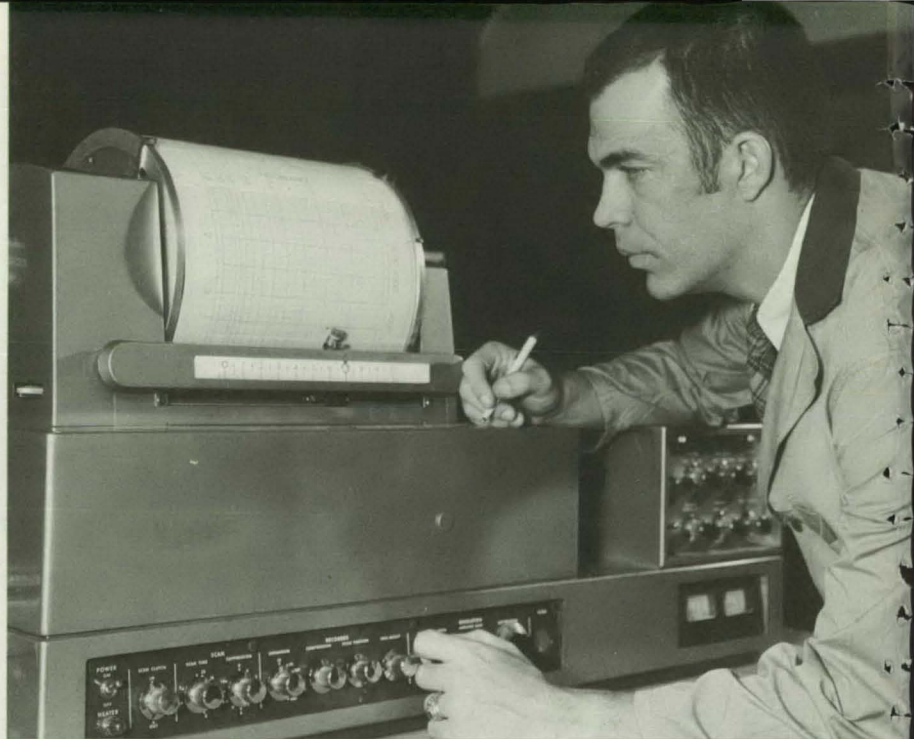
Using the infrared spectrophotometer, an examiner may identify and compare the organic components in paint.
