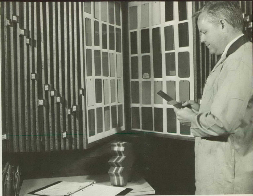
By reference to the panels in the National Automotive Paint File, the Laboratory examiner can often associate a paint chip with a particular make car.
