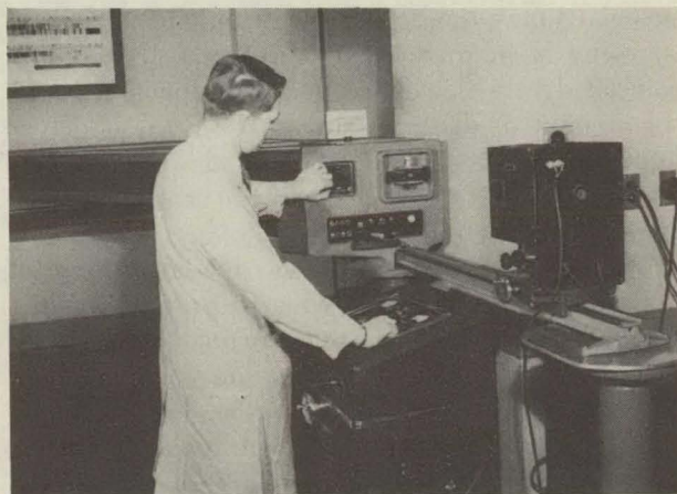
Figure 1.—Burning toxicological specimen on the grating spectrograph.
