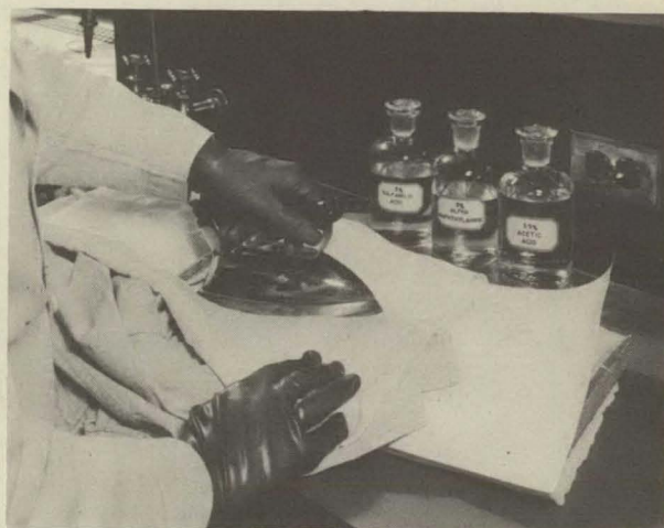
Figure 5. —Pressing the acetic acid dampened rag over the garment to be tested on an ironing board. The paper has been desensitized with photographic hypo; washed and dried; soaked in 0.5 percent sulfanilic acid in water solution and dried; then, soaked in 0.5 percent alpha naphthylamine in methyl alcohol solution and dried.
