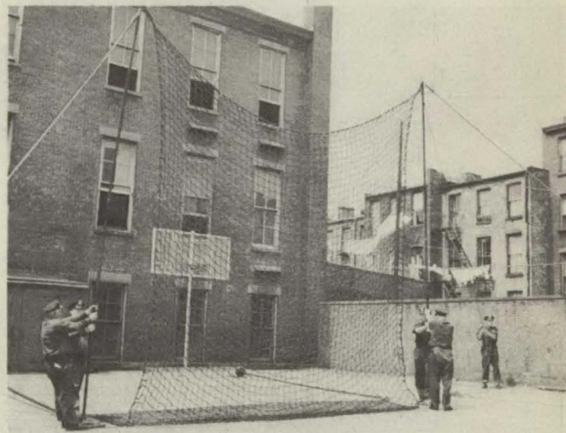
Figure 9.—Ground net being raised in sections by half of the crew.
