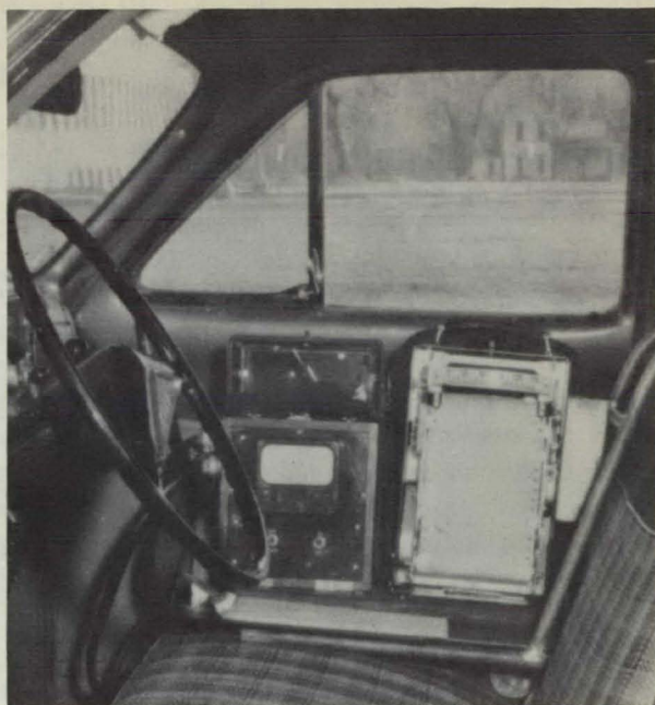
Front seat of radar car showing positions of the speed meter and the recording graph.
