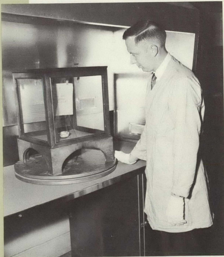
Iodine fuming cabinet in use.
