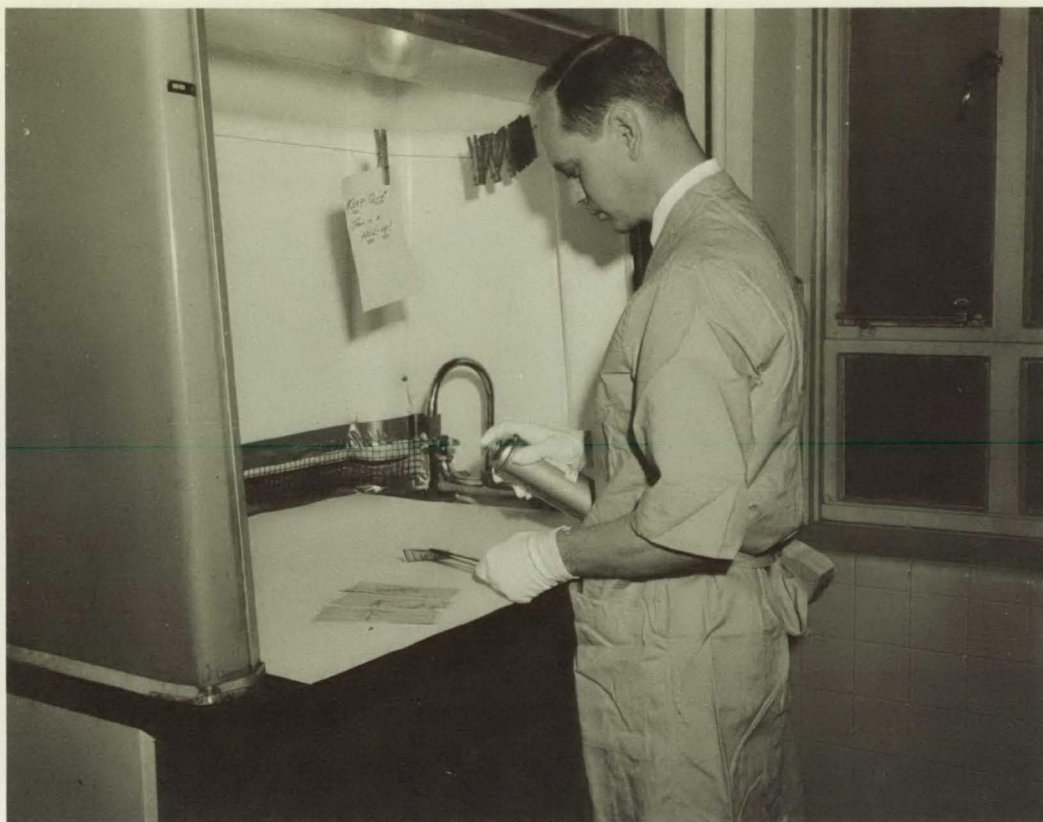
Ninhydrin solution being applied under an exhaust hood.
