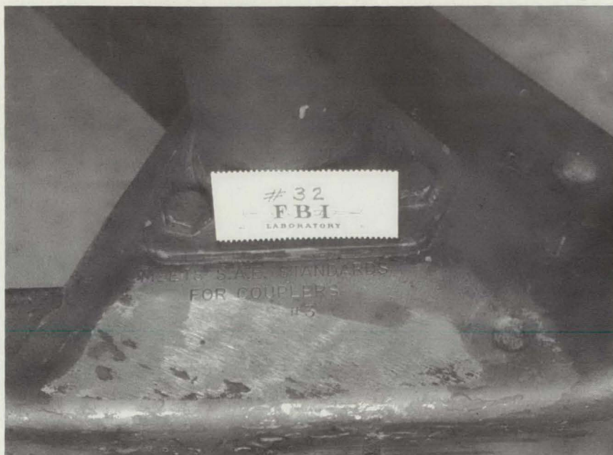
Paint remover uncovers ground-off serial number on trailer hitch.
