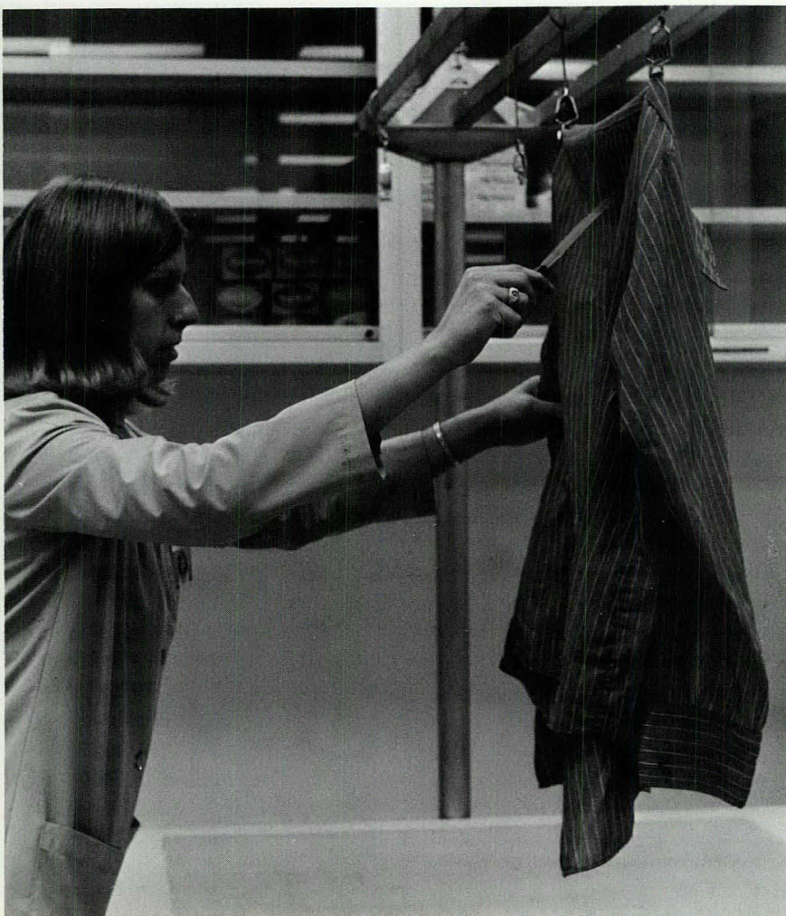
Laboratory technician uses metal spatula to scrape debris from surface of garment.
