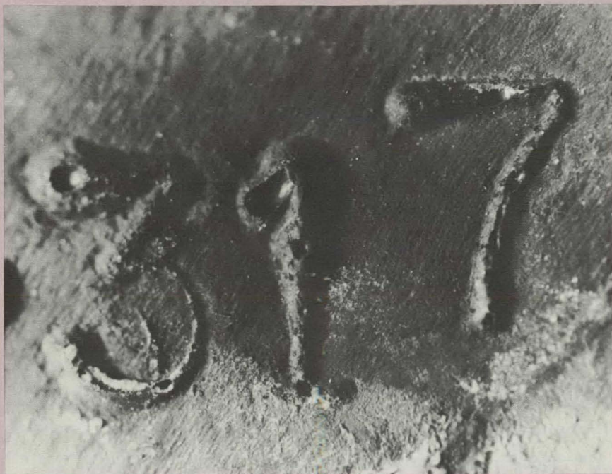
Figure 1 is an example of a cast VIN that is worthless for toolmark comparisons.
