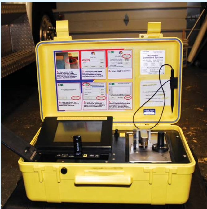
HazMat ID system with a USB drive inserted into it. This system can identify thousands of different substances, and the results can be downloaded onto a USB drive.
