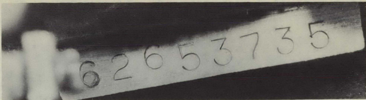
Closeup of altered 1951 Buick motor number. Note absence of factory mill marks.
