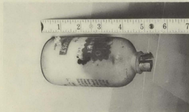
Cotton-packed plastic bottle used effectively as a gun silencer. One end of the metallic cylinder can be seen protruding from the bottle.
