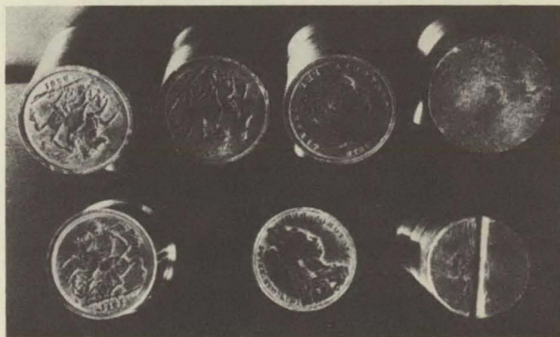
Figure 7. —Steel dies of English gold pounds. Apparently they were made by pressure rather than engraving due to the slight depth of the images.
