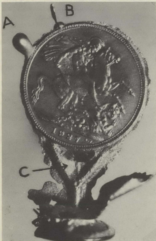
Figure 8. —A pound showing defects due to the expansion of the mold because of high temperature: "A" projection created by the melted gold remaining in the funnel-shaped groove in the mold; "B" projection created by the vent in the mold; "C" overflow of melted gold due to high temperature.
