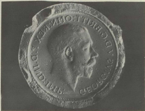
Figure 10.—Plaster mold of genuine pound after drying and removal from frame.
