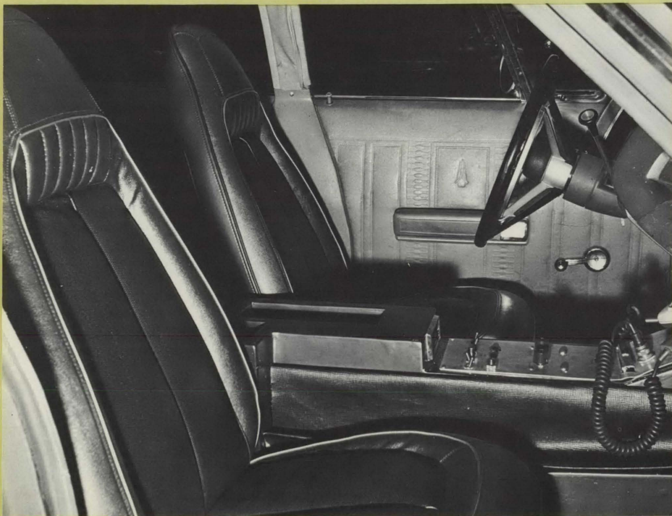
These individually adjustable seats and a center-mounted control console are the main modifications of the patrol car now being tested by the Detroit Police Department.
