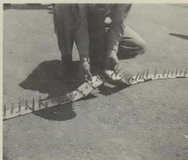
Figure 4.—Damage caused by car speeding over device with locked brakes.
