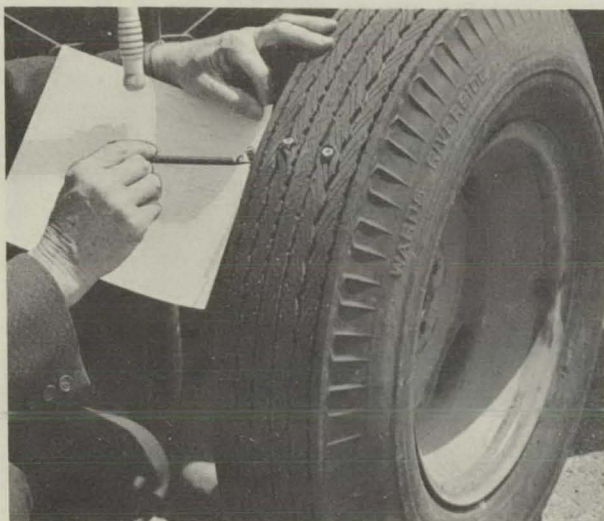
Figure 2.—Spikes imbedded in tire.
