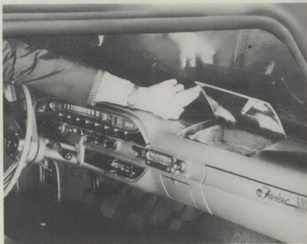
Fiberglass-lined compartment opened by switch hidden under instrument panel.
