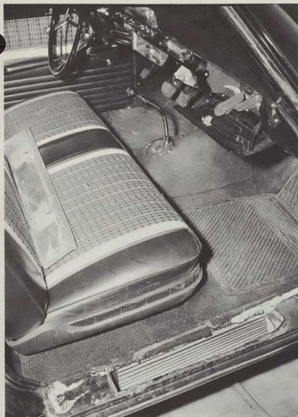
Floor-mounted transmission lever and secret doorsill compartment.
