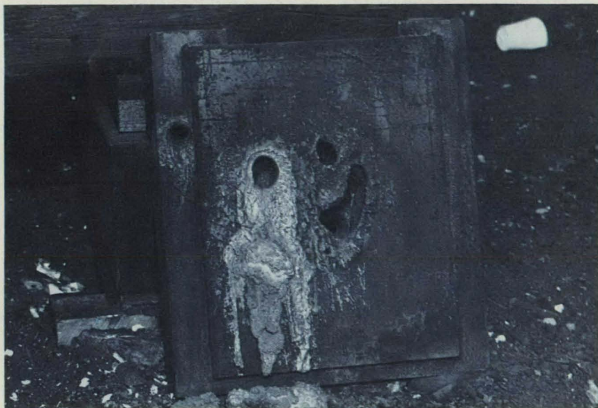
In a matter of seconds the thermal bar can burn through tempered steel. The above holes were made during a demonstration to test the burning power of the bar.
