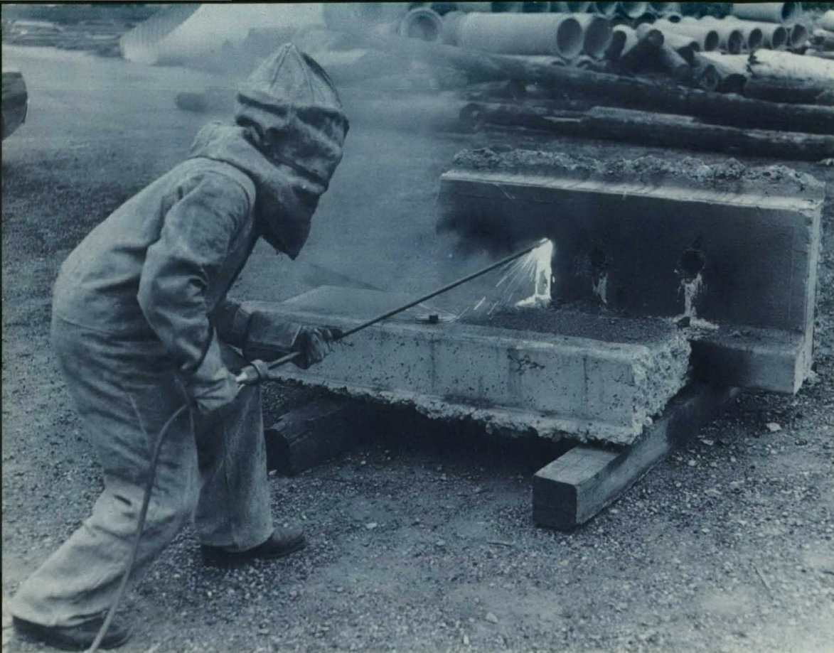
A demonstration shows how easily the bar can burn a hole in concrete.
