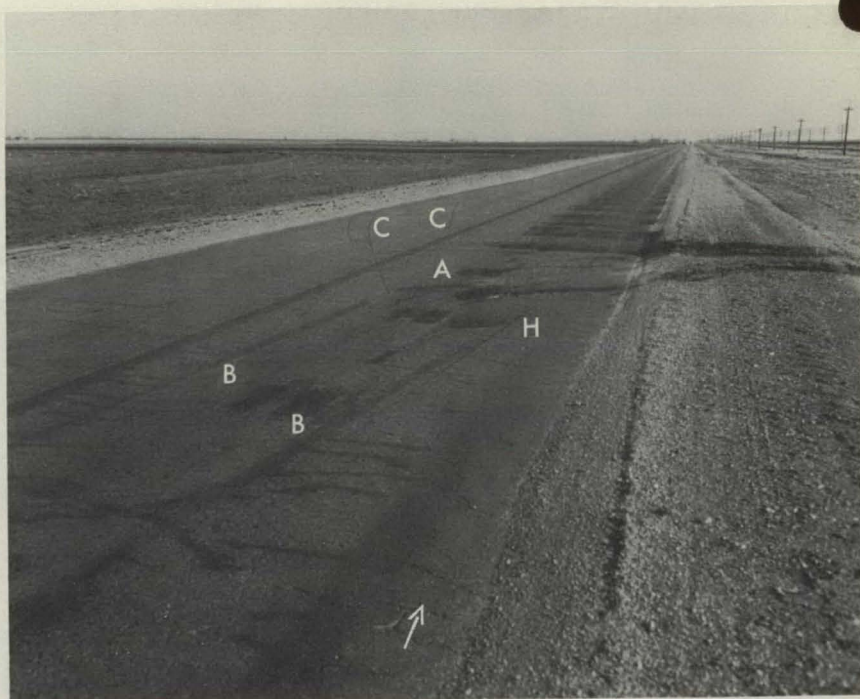
Exhibit 8: Point A marks gouges and spatter at collision point in Case E; B points out approach skidmarks of Unit 2; and C indicates approach yaw marks of Unit 1.
