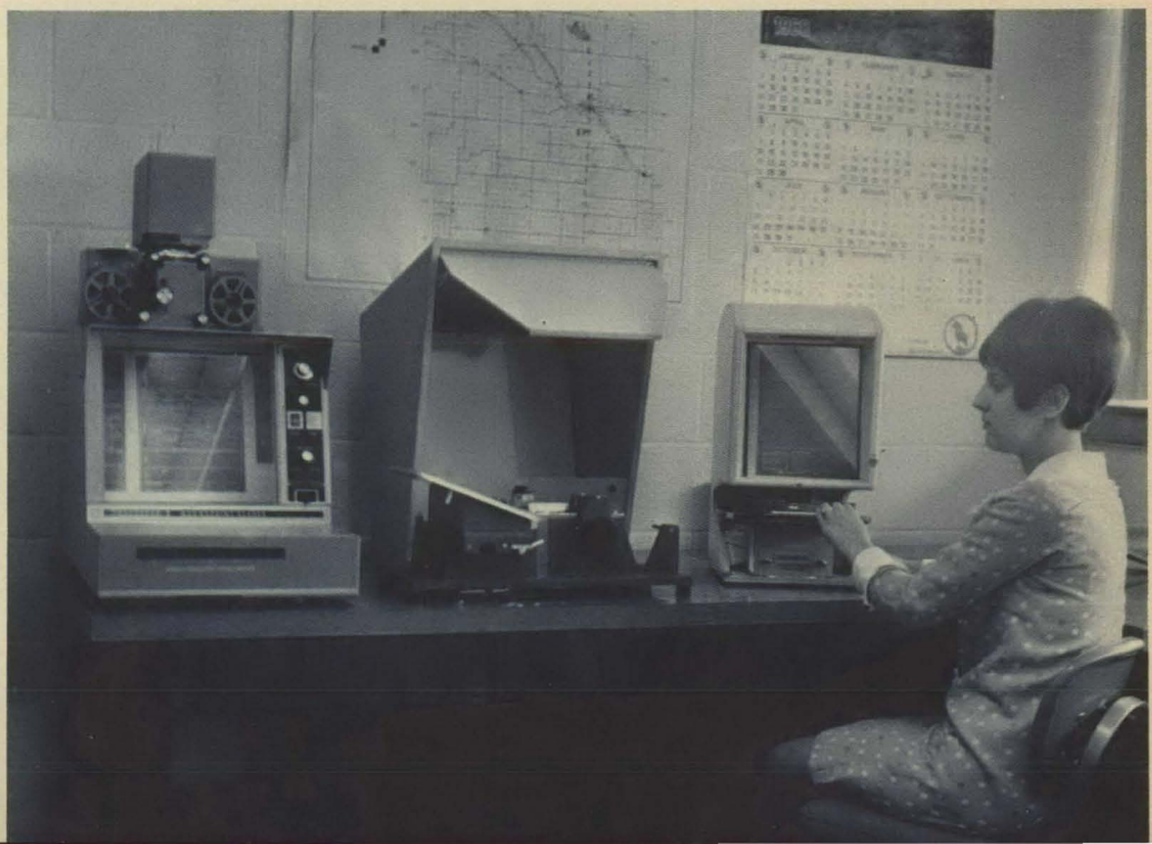
Machines purchased for the microfilming process included (left to right) a reader-printer, a jacket-filler, and a jacket-reader.
