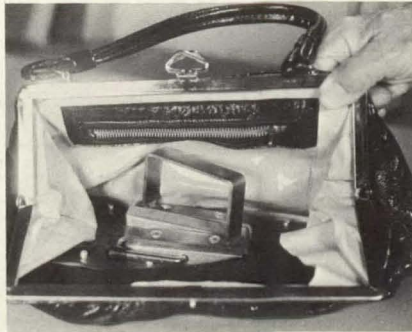
Suction-cup device can be activated by a lever inside the purse.
