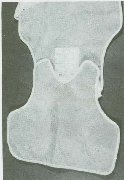
Inside of the body armor garment which was struck twice with a .38-caliber bullet, no penetration.
