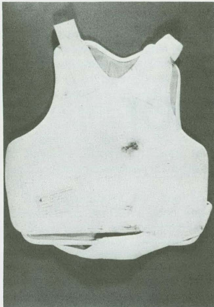
Two points of impact of .38-caliber bullets—one is to the right of center (note powder burns), the other is in the upper left area.
