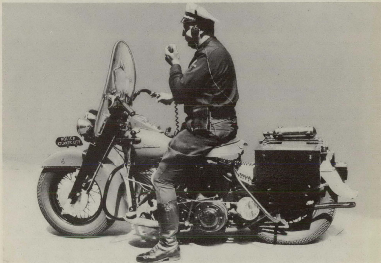
A motorcycle patrolman equipped with miniature two-way radio receiver and transmitter. A flexible antenna is worn over the shoulder.
