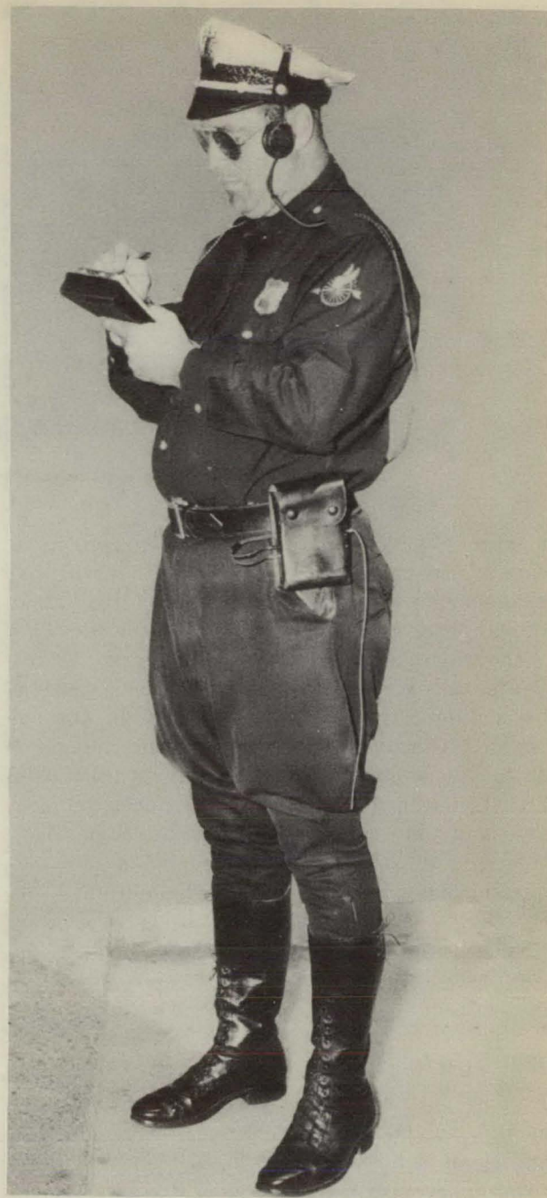
A motorcycle patrolman using the miniature receiver (belt type) away from the cycle.
