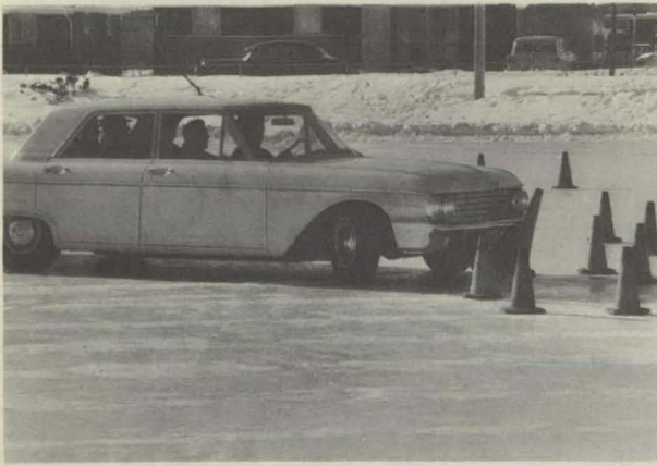
Improper right turn at too fast a speed causes front-end drift and a rear-wheel slide.
