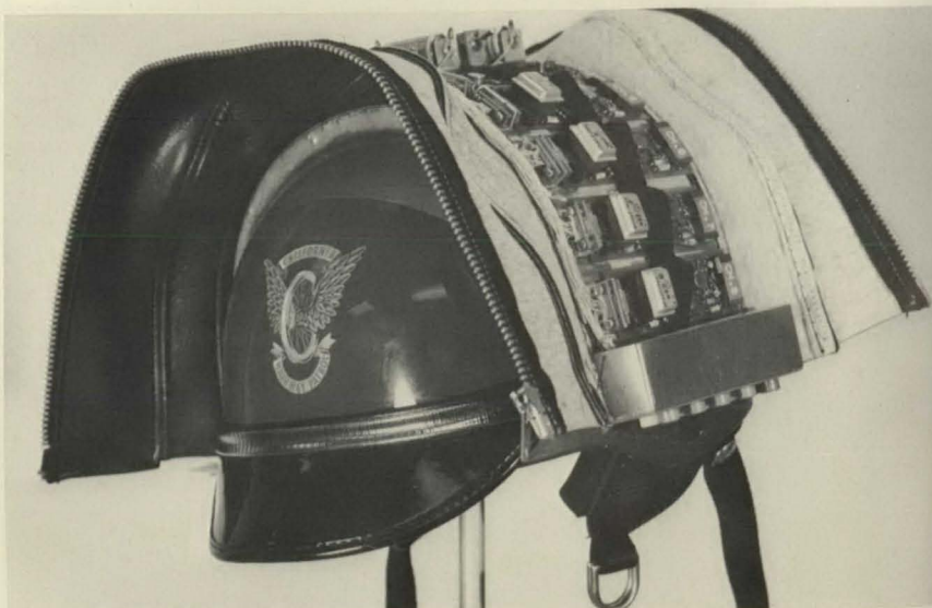
The special helmet used in the driver performance study transmitted information relative to the driver's physiological responses to recording devices.
