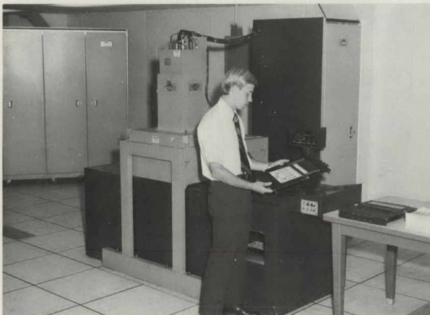
OPERATOR LOADING CARD HANDLER. THE SCANNER IS LOCATED OVER THE CARD HANDLER, SCANNER ELECTRONICS UNIT IS ALONGSIDE, AND THE PREPROCESSOR IS IN THE BACKGROUND.
