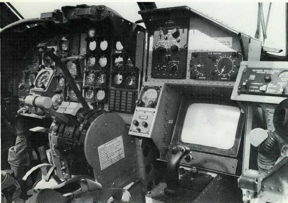
Sophisticated electronic equipment in the cockpit of a Customs surveillance aircraft includes a Forward Looking Infrared Sensing Device (FLIR).
