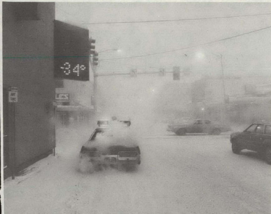
At extreme temperatures, moisture as expelled by heating units or vehicle exhaust crystallizes and is suspended in the air giving a unique manmade "ice fog." Traffic hazards that are present in any fog situation are only compounded by the cold.
