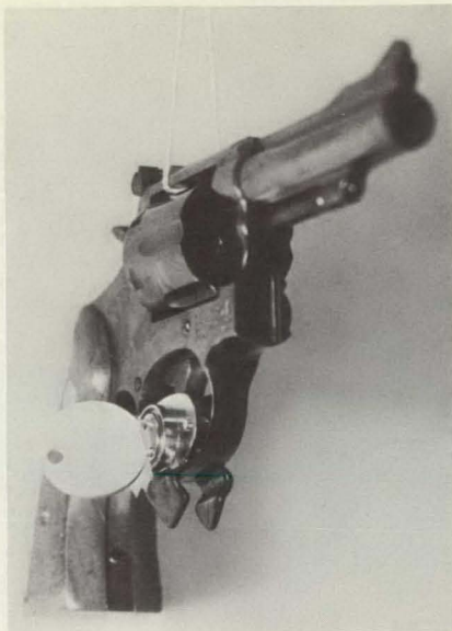
The locking device screws on the trigger housing and prevents the gun from being fired.
