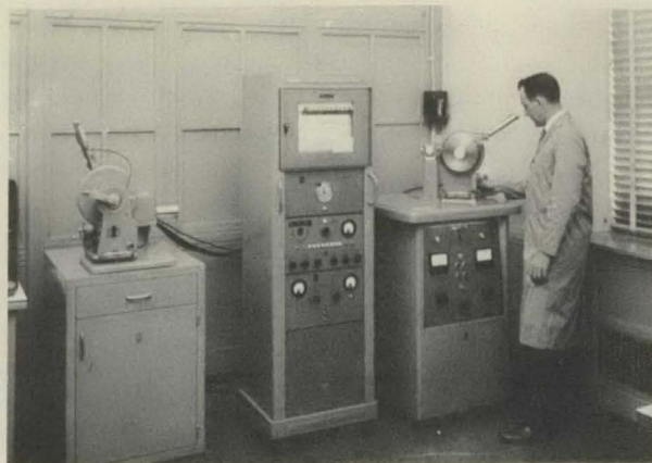
The X-ray spectrograph and diffractometer shown above are particularly useful tools in forensic chemistry where samples are often very small and must be subjected to nondestructive examinations.
