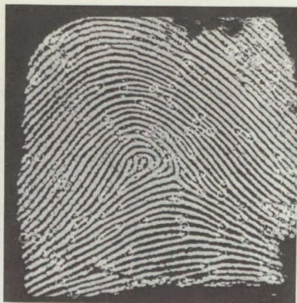
Figure 8.—An enhanced fingerprint as seen on the operator display scope of the system with each recorded minutia indicated by a small white circle.
