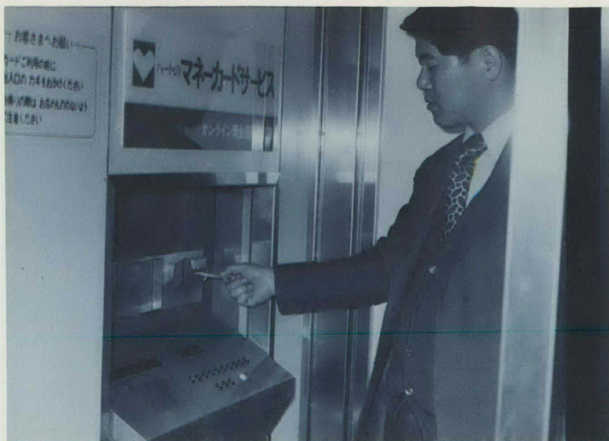
Money card is inserted (above) in automatic cash-dispenser station which issues currency (below) in the amount requested after the computer authenticates the transaction and the adequacy of the account from which the funds are to be withdrawn.
