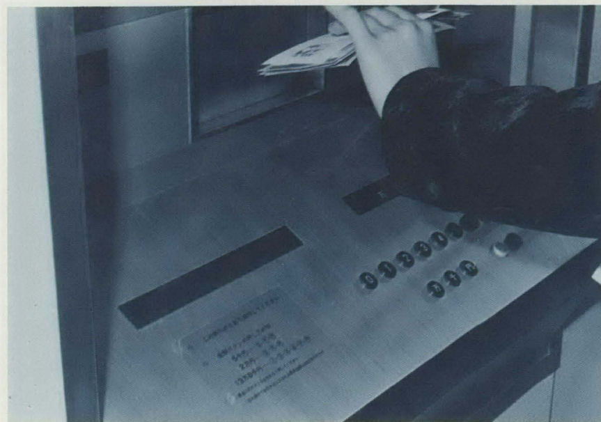
Money card is inserted (above) in automatic cash-dispenser station which issues currency (below) in the amount requested after the computer authenticates the transaction and the adequacy of the account from which the funds are to be withdrawn.
