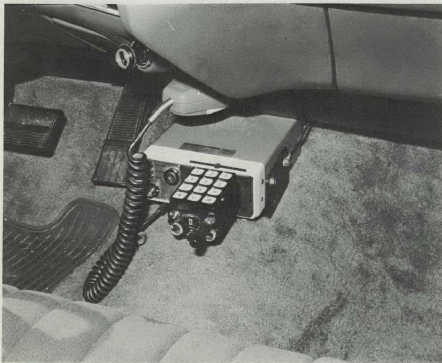
A view of in-car installation of the mobile/portable unit with the 12-button, touch-tone encoder clearly visible.
