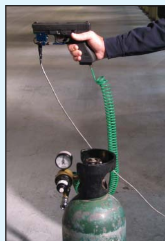
The air-recoil system, applicable for both live and dry fire, simulates recoil and resets the trigger for use in a classroom environment.
