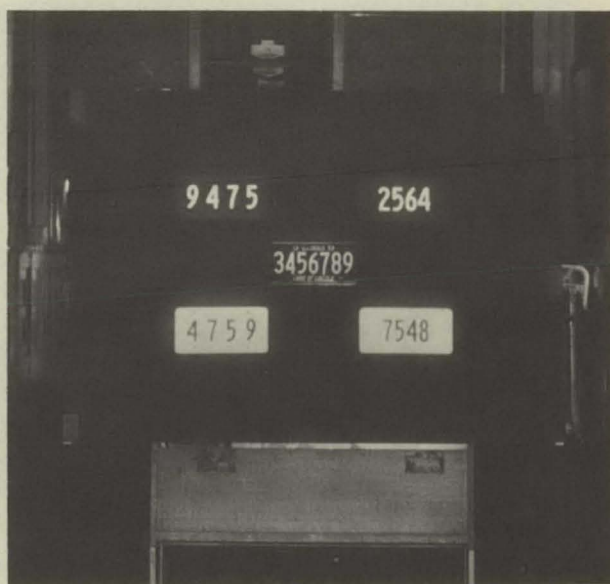
Figure 5.—Some reflectorized license plates from this study compared to the present Illinois nonreflectorized license plate. The reflectorized plates are shown with two contrast directions and at two different spacings of the digits.
