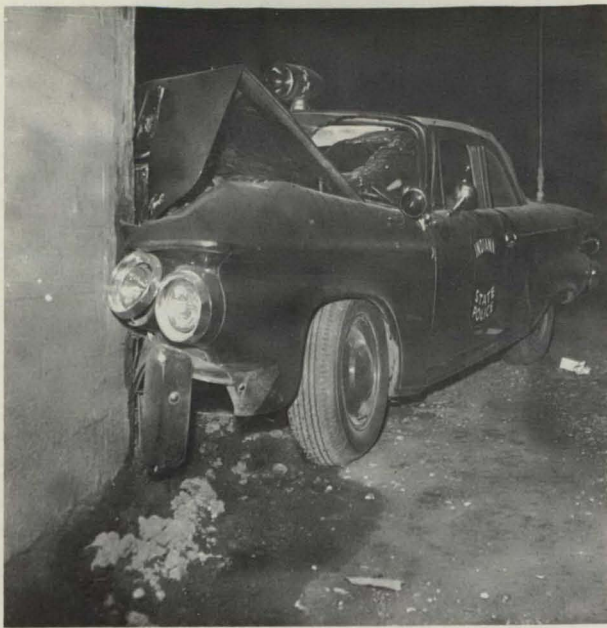
The trooper smashed into the concrete bridge pillar at 60 miles per hour. Because he had fastened his safety belt, he suffered only minor injuries. The force of impact shoved the engine 1½ feet backward.
