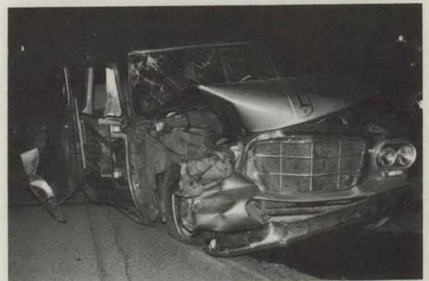
The driver of this car suffered a minor laceration on his chin after hitting a stalled vehicle at a speed of 55 miles per hour. The driver credited his snugly fastened seat belt with preventing more serious injury.
