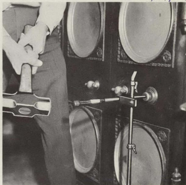
Punch held firmly in place ready to be struck by the sledge hammer.
