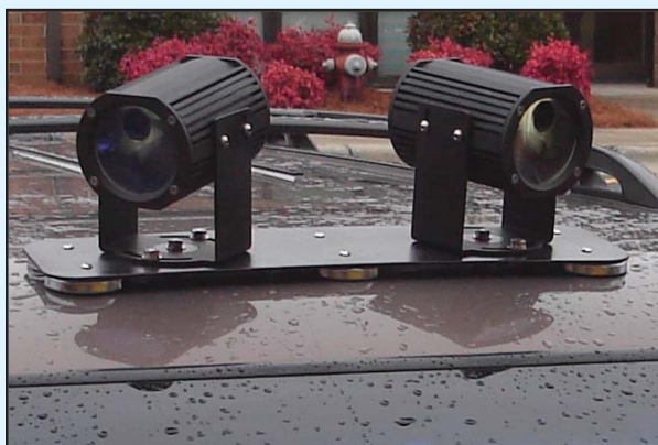
Mobile LPR unit temporarily attached to vehicle's roof.
