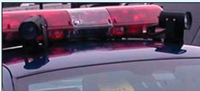
LPR unit installed onto cruiser's light bar.
