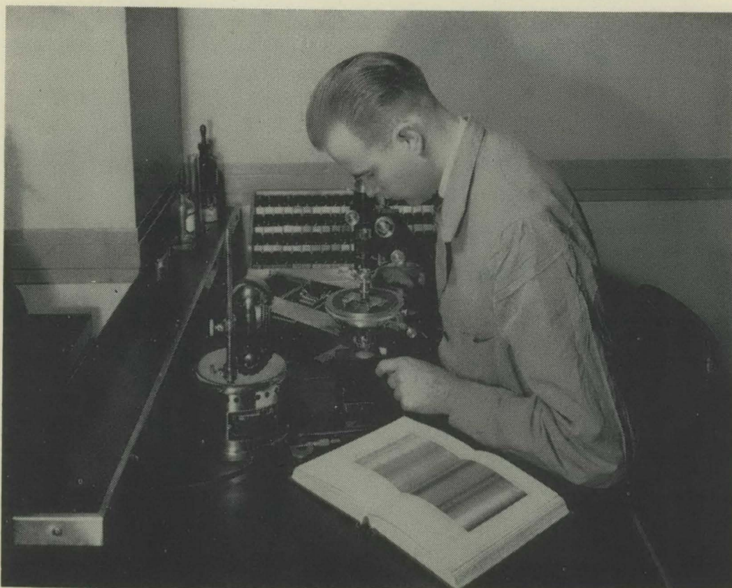
ONE OF THE FBI EXPERTS EXAMINING EVIDENCE THROUGH A PETROGRAPHIC MICROSCOPE
