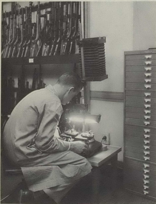
An examiner using one type of comparison microscope available to the experts in the FBI Laboratory.
