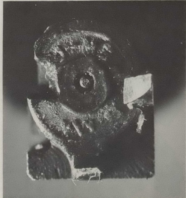
Impressions in grease on the breechface may provide the headstamp marking of the last cartridge fired.
