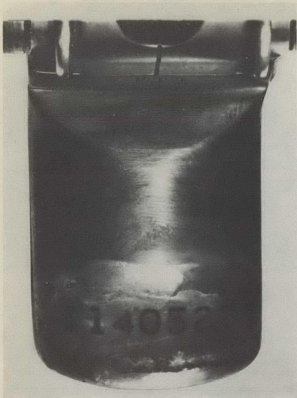
Restored serial number on a rifle.
