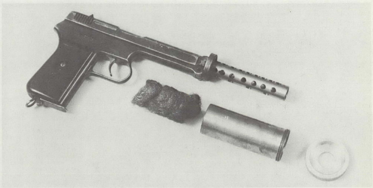
Figure 7. Internal Construction of a Typical Pipe Silencer. This device is welded to the muzzle of this 9 mm Browning Short (.380 ACP) caliber firearm of Czechoslovak manufacture. However, due to the large bore size of this device, it is not very effective.
