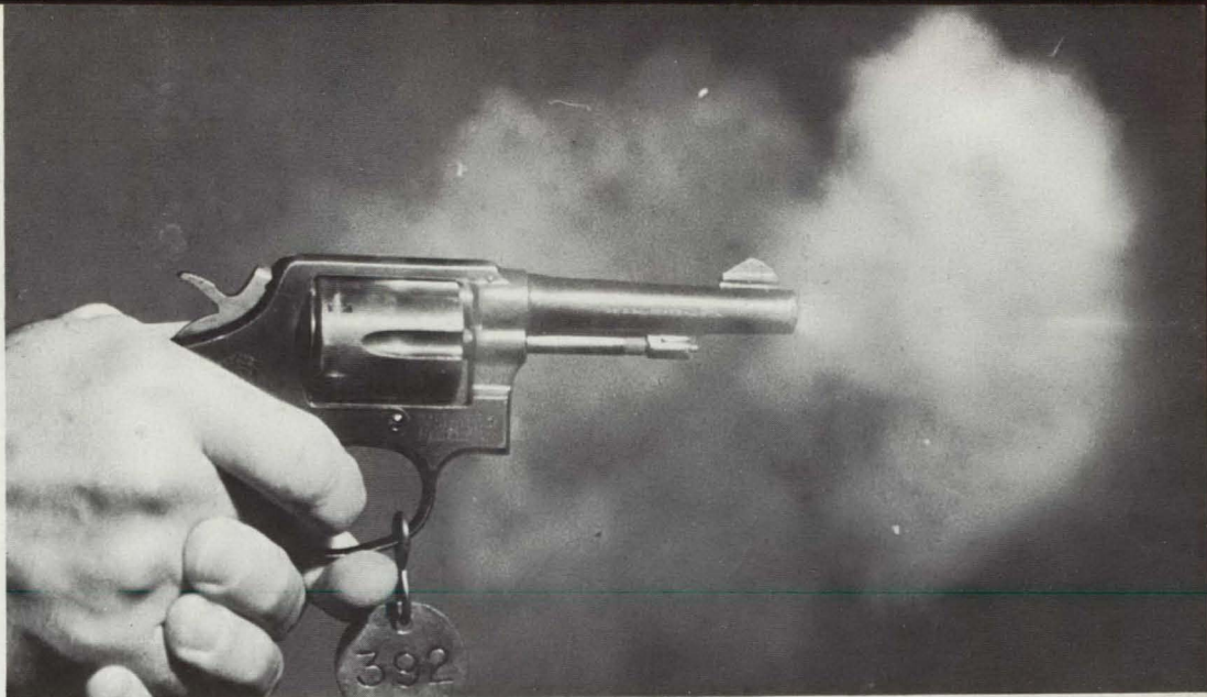
Figure 10. Gases Caused by Firing. Gases escape from a revolver at two places. The first escapage is at the juncture of the cylinder face and the barrel breach. The second is at the barrel muzzle. It can be seen that great amounts of gas escape at both points.
