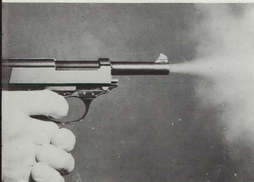
Firearm. The gases generated during the firing of a 9 mm parabellum (Luger) case a Walther, P-38, are voluminous, as can be seen here. This illustrates the sound pattern. The more gas control, the more sound control. (See fig. 3.)
