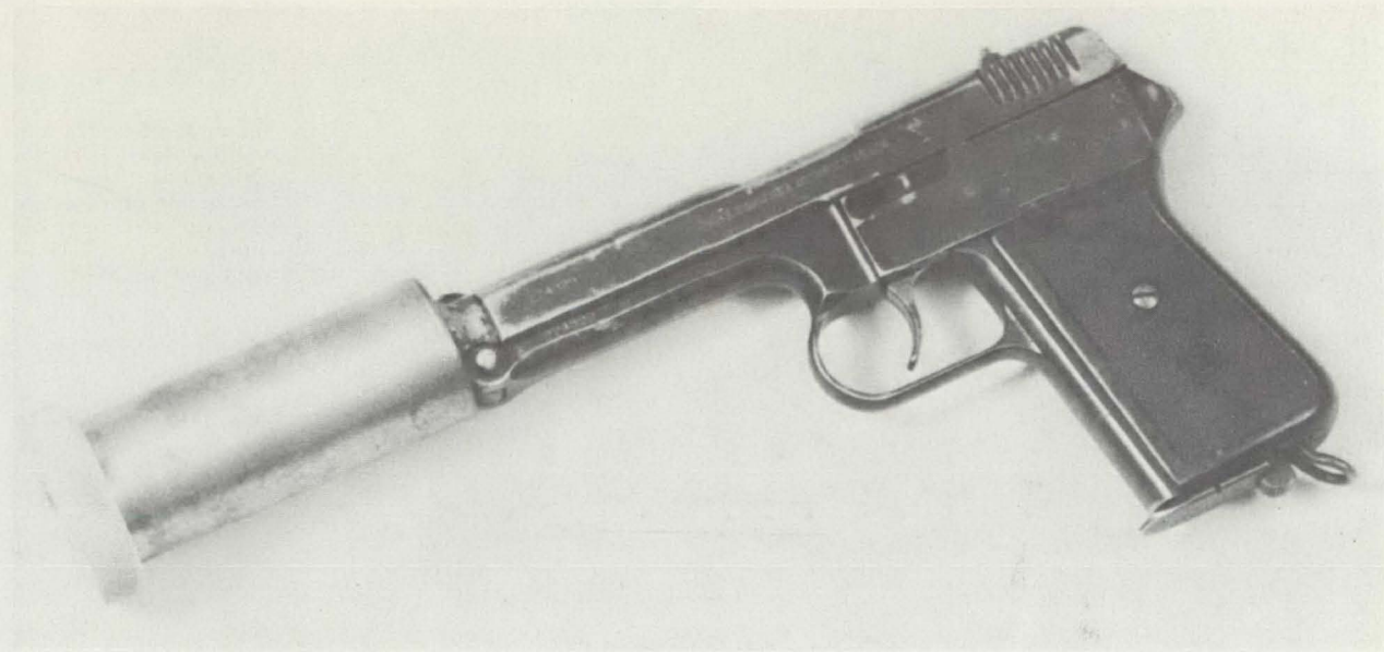
Figure 6. Pipe Silencer. Shown is a typical firearm silencer manufactured from a length of galvanized pipe. It is filled with steel wool, which is used as a gas absorbent. If the exit hole at the muzzle end of the device is of the proper size and the quantity of steel wool filler is sufficient, the silencer can be effective.
