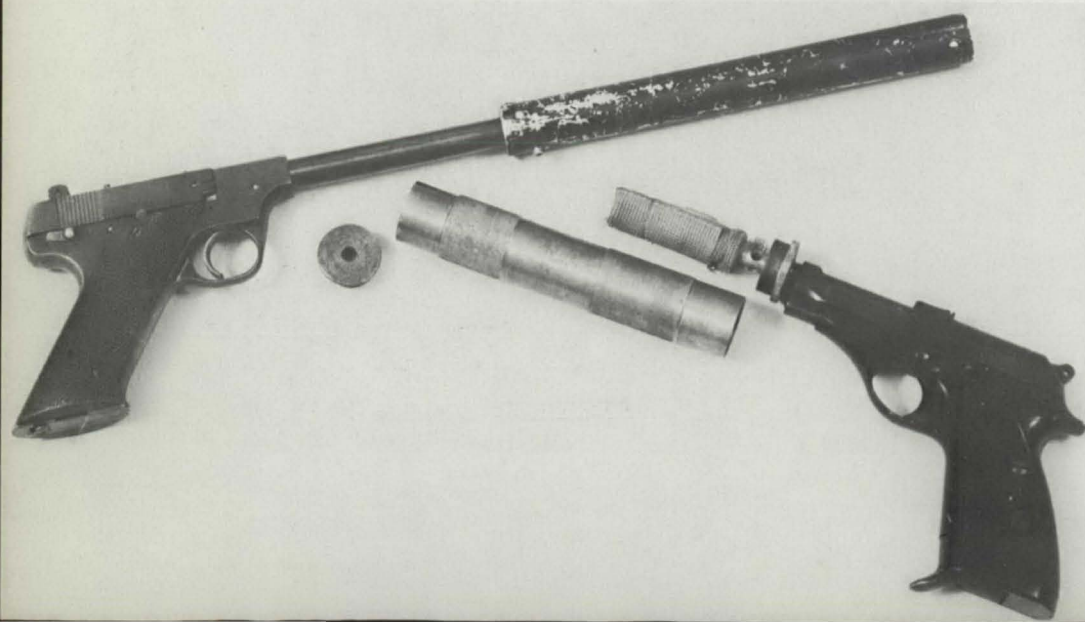
Figure 9. Internal Construction of a Typical Homemade Firearm Silencer. Although the internal fittings are quite simple, homemade silencers can be very effective. As illustrated here, a ported barrel extension, wrapped in screen wire mesh and surrounded by a closed tube, acting as an expansion chamber, is sufficient to reduce the sound level up to 30 dB.
