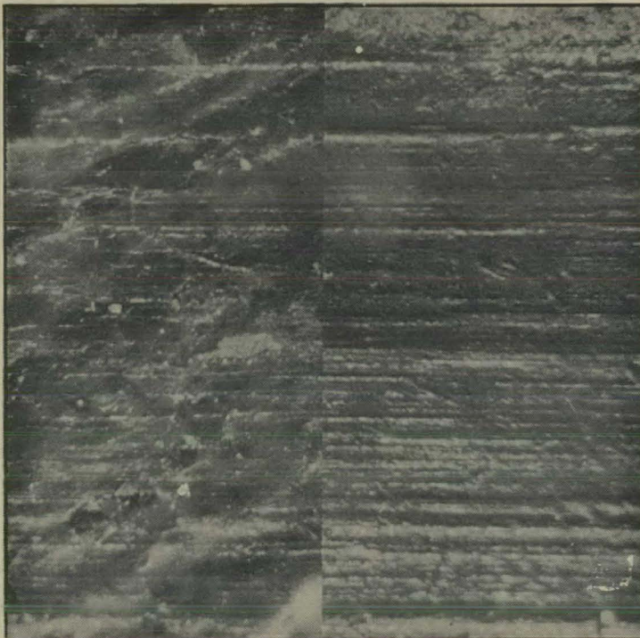
Photomicrograph showing comparison of markings found on the evidence with markings produced on test material with the suspected hammer.
