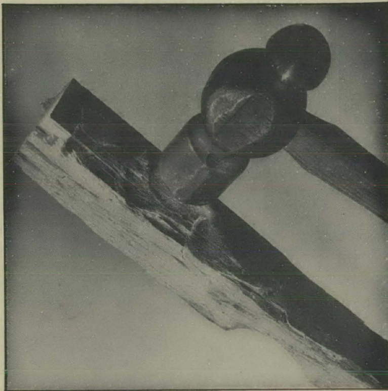
Position of hammer in striking wood as determined by alignment of markings produced on the wood.
