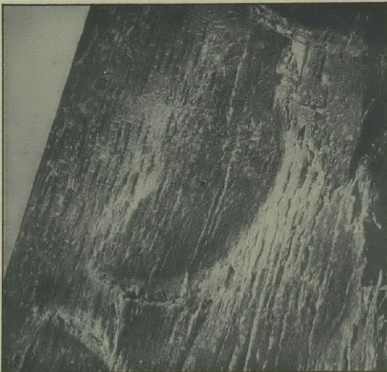
Striking surface of hammer showing irregularities.
