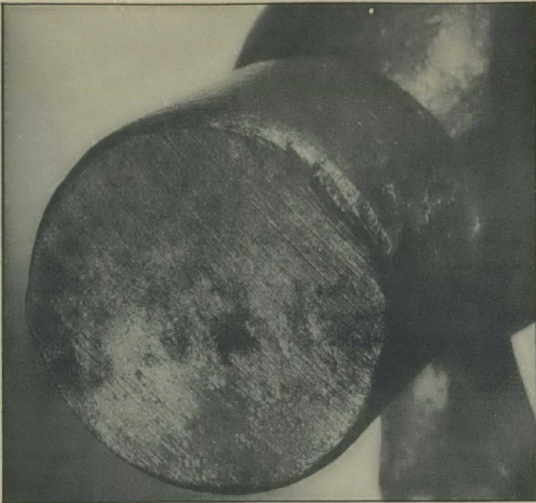
Striking surface of hammer showing irregularities.
