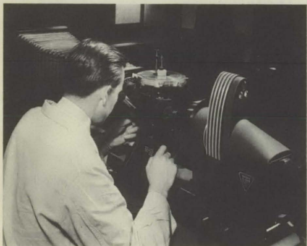
In the Metallurgy Unit, the metallograph is used to study the crystalline structure of metals.
