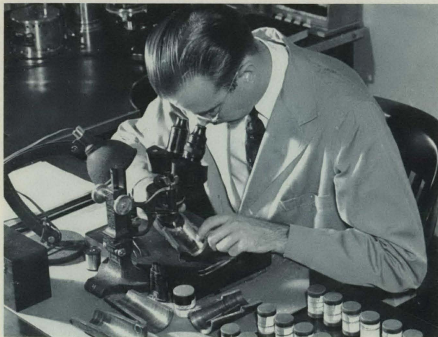
An examiner conducts a petrographic examination of an abrasive substance found in a motor bearing. Boxes at right contain abrasive specimens for comparison.
