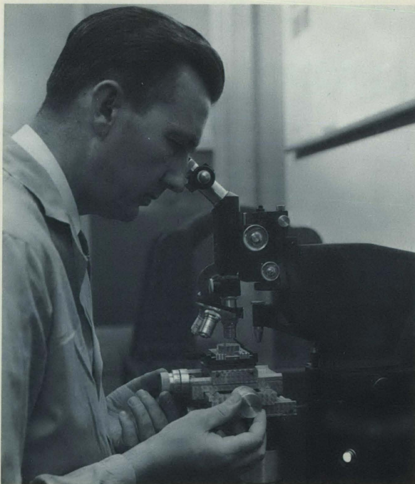
A Laboratory expert determines the hardness of small pieces of metal with the microhardness tester.
