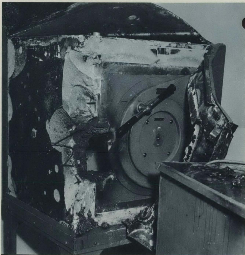
The burglar on this job first tried drilling the chest, then drifting and punching, and finally was successful when he ripped the safe and cut into it with a torch.
