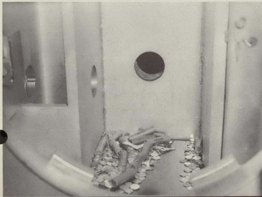
Diamond core bits were used to drill the holes in this safe through which valuables were taken.
