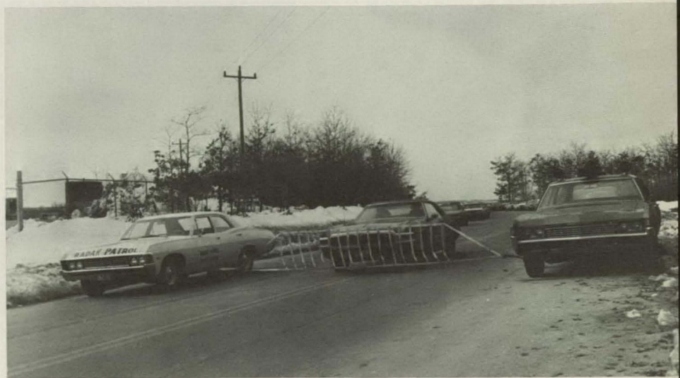
When a car moving at high speed strikes the net, the braking force is equally distributed over the front end of the vehicle.
