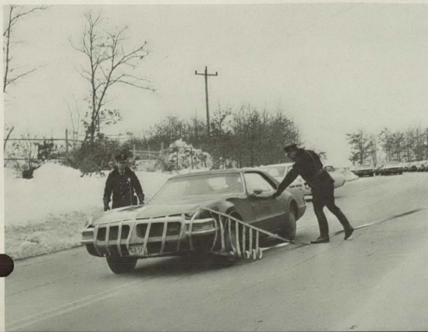
Damage to cars halted by the device has been minor, and no frame-bending or serious denting has occurred.
