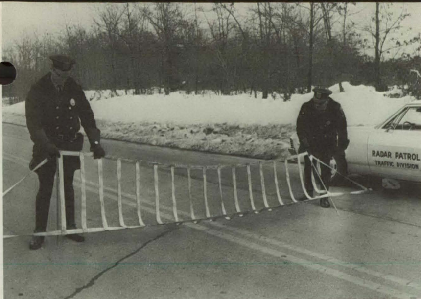
Energy absorbers are attached to each end of the nylon net and these in turn are connected to the anchors.
