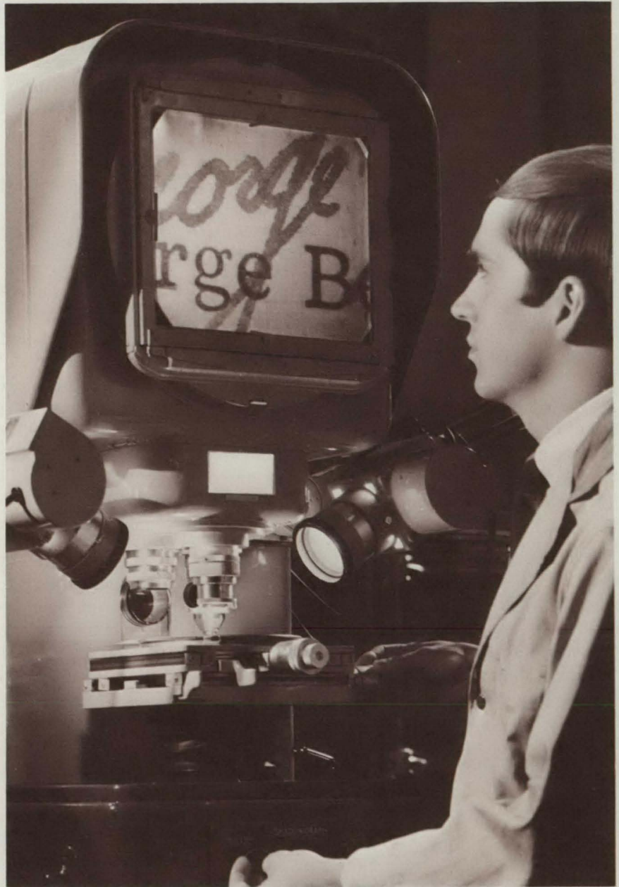
The shadowgraph shown is used to greatly enlarge document specimens.
