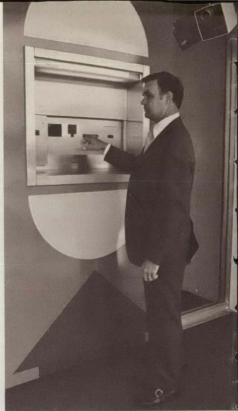
Automatic teller is capable of handling many types of transactions such as making deposits, dispensing cash, and transferring funds from one account to another—all without the services of a teller.
