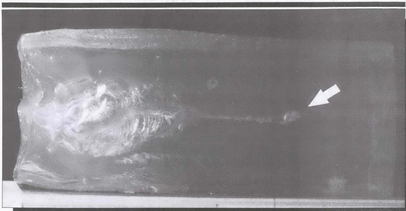
The side view of a bullet's track through a block of ballistic gelatin. The white arrow shows the location of the bullet.
