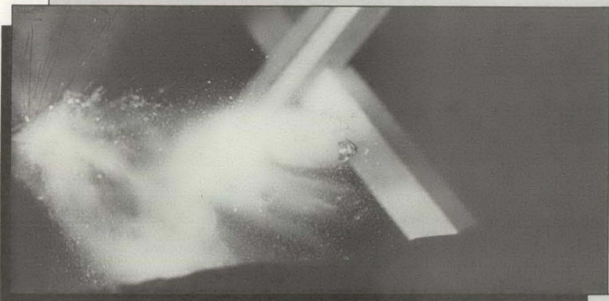
An ammunition test shot being fired into auto windshield glass.
