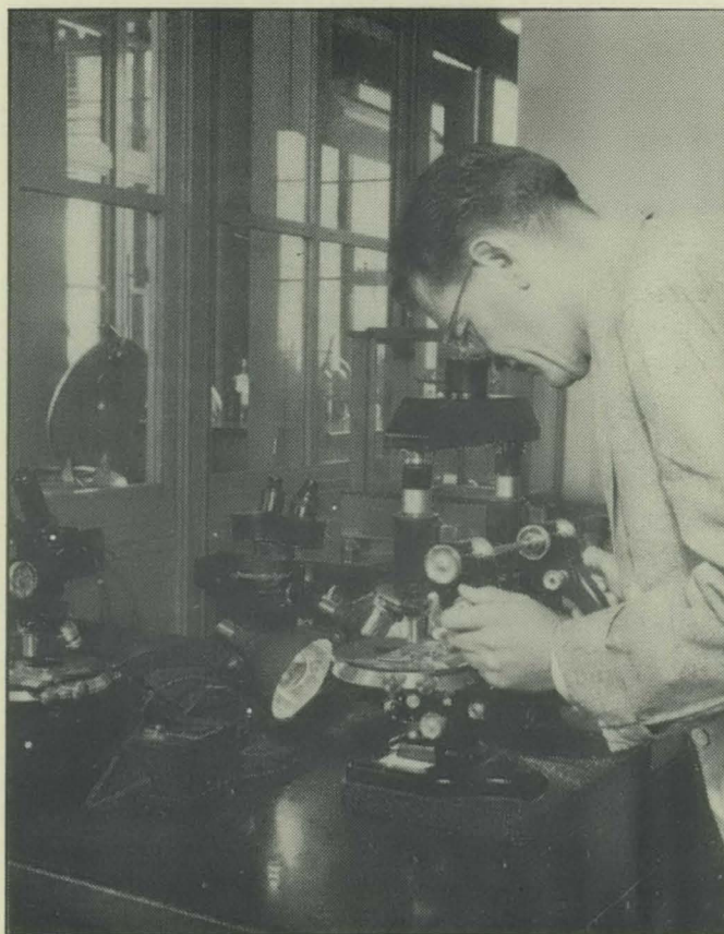
LABORATORY TECHNICIAN USING SPECIAL COMPARISON MICROSCOPE FOR FIBER EXAMINATIONS
