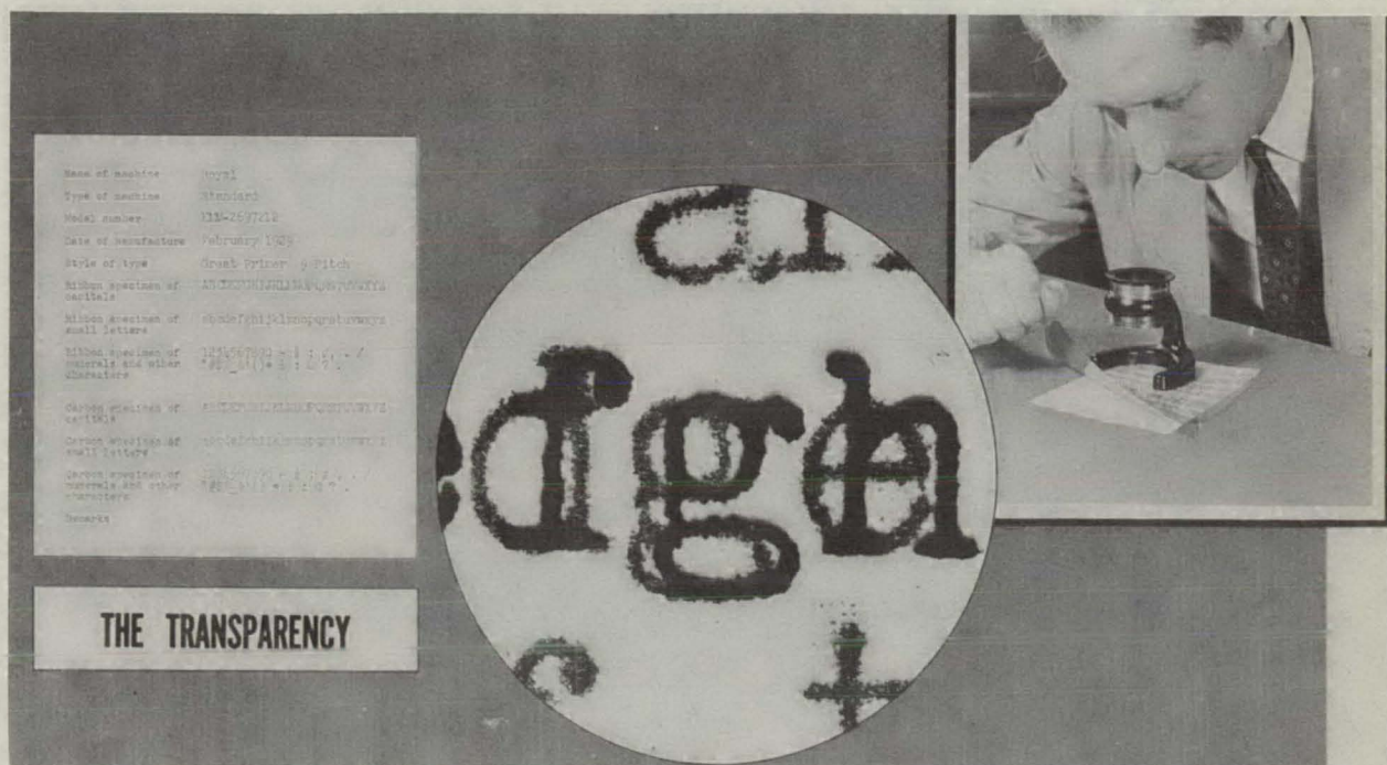
Figure 5. —Using a transparency to determine the make and model of typewriter. The “g” in the transparency is partly superimposed over the “g” in the document under examination.
