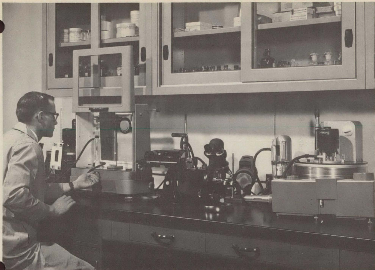
The above photograph shows a density measurement being made on the density balance. To the right of the balance are a precision refractometer, a microscope, various light sources, and a water bath. Thermostatically controlled temperatures are maintained by means of water circulating through the lengths of tubing seen in the photograph.
