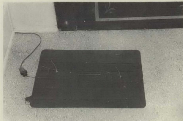
Wired rubber mat is placed on floor in front of vault. When stepped on, alarm is sounded.
