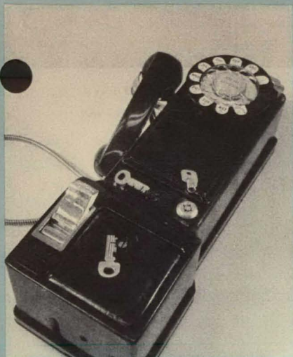
This is a 200 series coin telephone with the three locks and keys most commonly used. All keys are serially numbered and can usually be traced to place of issue and the employee to whom issued.
